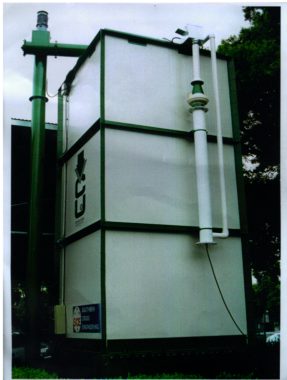
Plate 4 - Vertical Composting Unit
